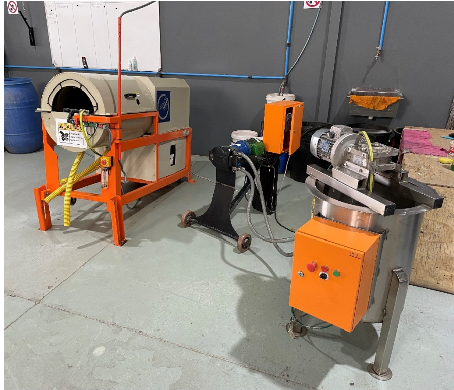
Figure 2: MGS C900 test unit, mixing tank and peristaltic pump that was used for the testwork
